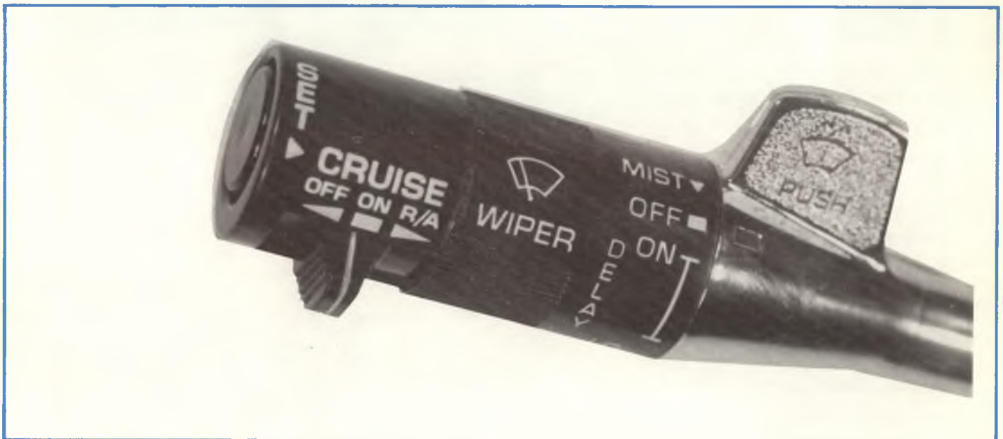
Figure 1-1, Mode Control Switches on Turn Signal Lever.
